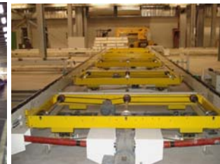
Handling system on skid
