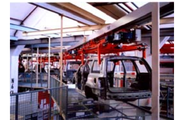
BiW Shop - Overhead TTS
